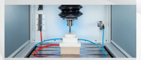
Precise electro-chemical machining (PECM) is the ideal process for the non-contact, almost wear-free machining of workpieces made of high strength materials such as nickel-based alloys. At IMTS, EMAG will have displays demonstrating the PECM system and its effectiveness in machining extremely difficult 2D and 3D contours. Experts in ECM and PECM will be available to discuss production challenges or opportunities first-hand.
