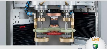
The MIND-M 250 induction hardening machine offers a high degree of precision and reliability with comparably low investment costs. Simple heat treatment tasks, such as annealing or induction hardening, with a maximum power requirement of 100 kHz in high frequency (HF) or 30 kHz in medium frequency (MF) applications can be processed with the MIND-M 250
